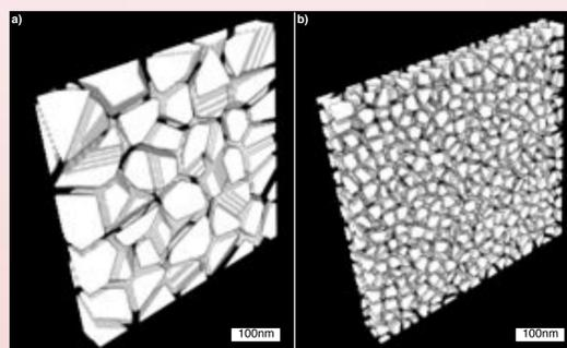
**Fig. 3.** Three-dimensional representations of the CZ used to simulate the holography results. The dimensions of the islands and matrix match those observed experimentally.
