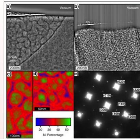
**Fig. 2.** STEM images of (a) course and (b) fine regions of the CZ (bright = tetraenaite, dark = matrix). (c, d) Composition maps of the intermediate CZ with islands 50%Ni:50%Fe and matrix 25%Ni:75%Fe. (e) Diffraction pattern representative of both the coarse and fine CZ.
